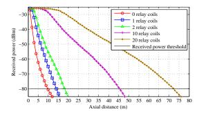
Fig. 2. Received power of a 10 MHz+0.5 KHz signal using MI waveguides with different relay coil numbers.
