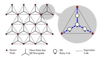
Fig. 3. The MI waveguide deployment using TC algorithm in the WUSN with hexagonal tessellation topology.
