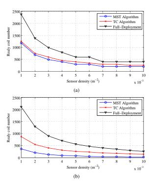
Fig. 5. The number of relay coils to connect 100 sensors in WUSNs with (a) hexagonal tessellation topology and (b) random topology.
