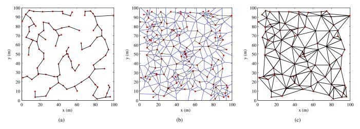
Fig. 6. The deployment results of (a) the MST algorithm, (b) the TC algorithm, and (c) the full-deployment strategy. (The red dots are the sensors; the black lines represent the MI waveguides; and the blue cells are the Voronoi diagrams. 100 sensors are uniformly distributed with of a spatial intensity  $\lambda_{rand} = 0.01 \ m^{-2}$ .)
